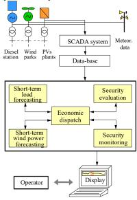
Figure 1: The control system architecture.
