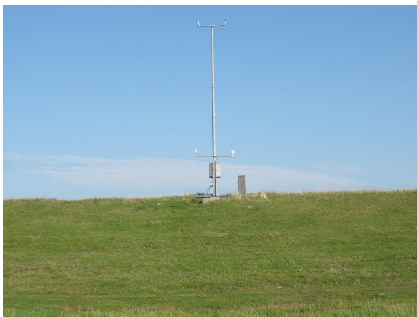
Figure 3.1. A synoptic weather station (WMO 06090). Instruments for measuring wind speed and direction are located on the 10-meter boom. Instruments for measuring temperature, humidity and global horizontal irradiance (GHI) are located on the 2-meter boom. At other stations GHI is measured on a separate post.
