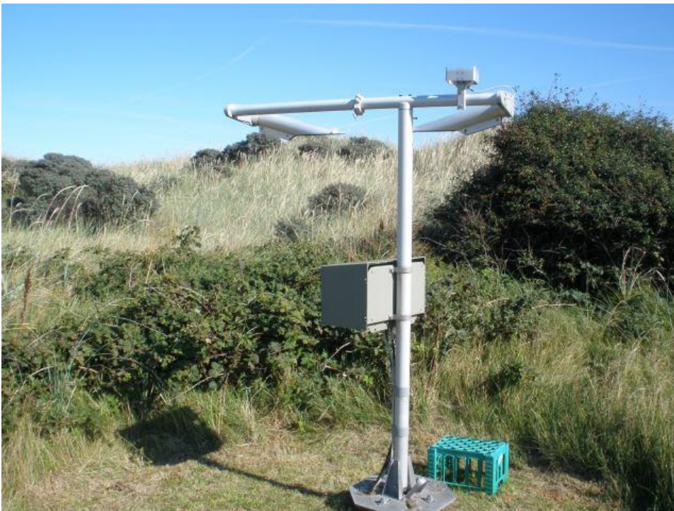
Figure 3.2. A forward scattering visibility meter (WMO station 06041).
