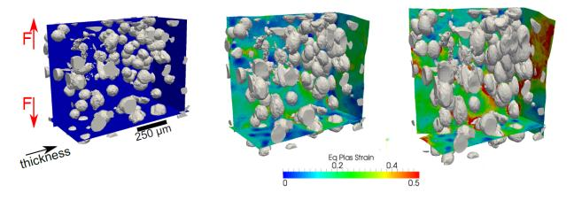
**FIGURE 4.** ROI calculation results using the DVC-FE approach and showing void growth and plastic strain for three different states during the tensile test.
