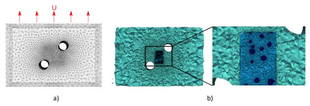
**FIGURE 3.** a) Mesh used at the specimen scale for the w-FE approach and b) inside view of the mesh used for the s-FE approach with detailed view of the heterogeneous ROI.
