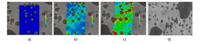
**FIGURE 5.** a), b) and c) Superposition of strain fields and X-ray laminography pictures at different stages of loading. d) Final coalescence mechanisms.
