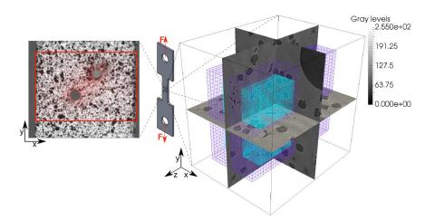
**FIGURE 2.** Schematic view of the sample with the definition of DVC (blue) and FE (cyan) meshes plotted over the corresponding cast iron microstructure in isometric view [10]
