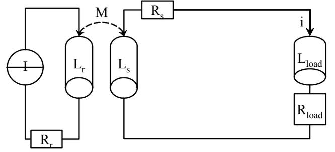
**Figure C.1 Equivalent lumped circuit for the power system. When the rotor is made to rotate at a constant speed (primary), the three phases (secondary) experience a periodically varying magnetic field. Here they are gathered thanks to a Park's transformation [28].**
