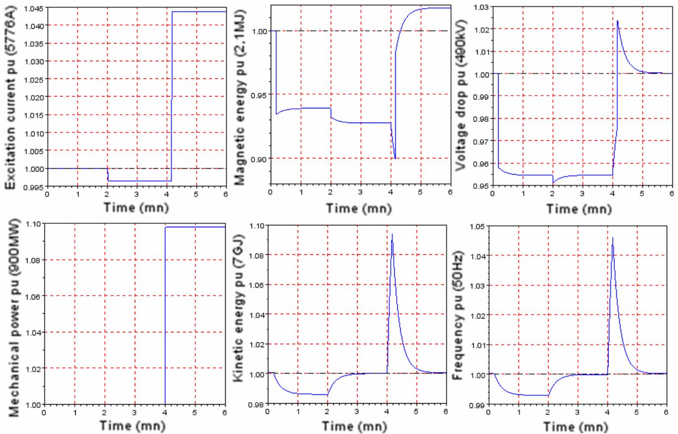
**Figure 4 Behavior of the kinetic and magnetic reserves under fluctuation and control. Calculations are made thanks to a time-stepping integration of (appendix C.1) with a resolution of the phasor diagram (appendix C.2) at each time step. The rated values refer to appendix C Table 1.**
