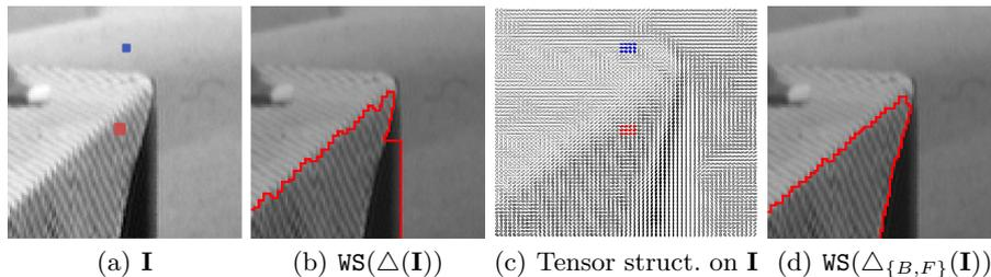
**Fig. 1.** (a) Red and blue squares show the pixels of sets  $F$  and  $B$  respectively. Image (c) is the representation of the structure tensor of the grey scale image (a). Pixels in  $F$  and  $B$  are coloured in red and blue. Image (b) is the marked based watershed on classical gradient, and (d) is the marked based watershed on supervised gradient.
