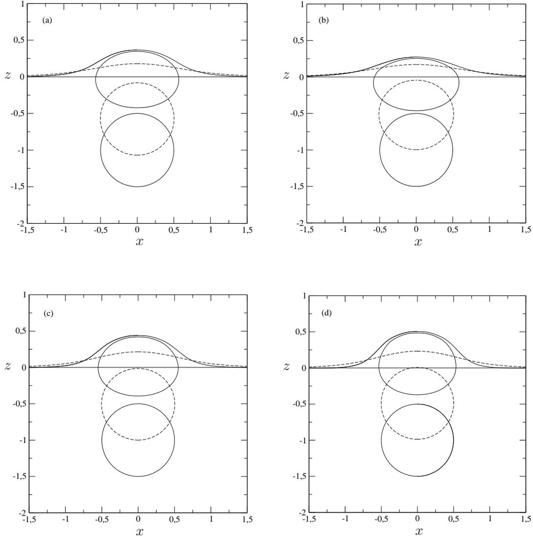
Figure 3: Bubble and free surface shape at  $Bo = 1$  for (a)  $\gamma_0/\gamma_1 = 1$ , (b)  $\gamma_0/\gamma_1 = 2$ , (c)  $\gamma_0/\gamma_1 = 0.5$  and (d)  $\gamma_0/\gamma_1 = 0.2$ . Dashed lines indicate the bubble and free surface shapes for  $t = 0.59$  while  $t = 1.746$  at finale stage.
