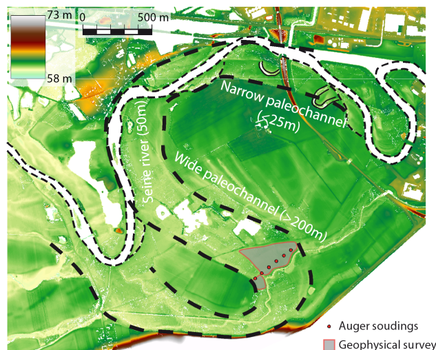
Figure 2. Lidar map of the study area, showing the contemporary location of the Seine River, together with the narrow and wide paleochannel interpretations.
