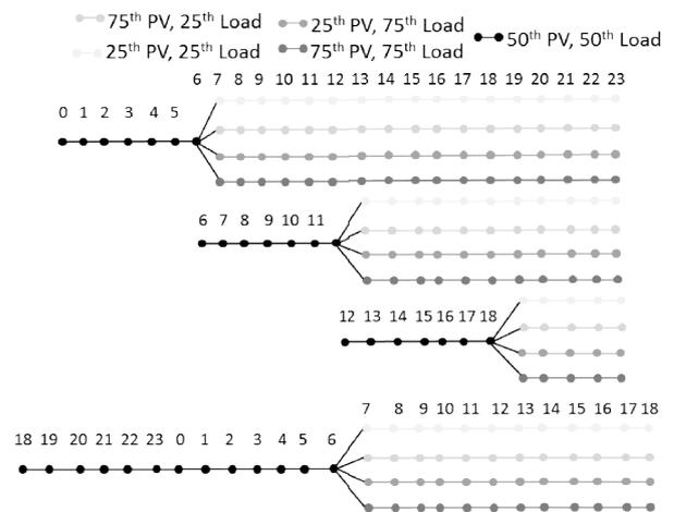
**Figure 2: Stochastic analysis with a four dimensional scenario tree using 25<sup>th</sup>, 50<sup>th</sup> and 75<sup>th</sup> quantiles of PV and load profiles**
