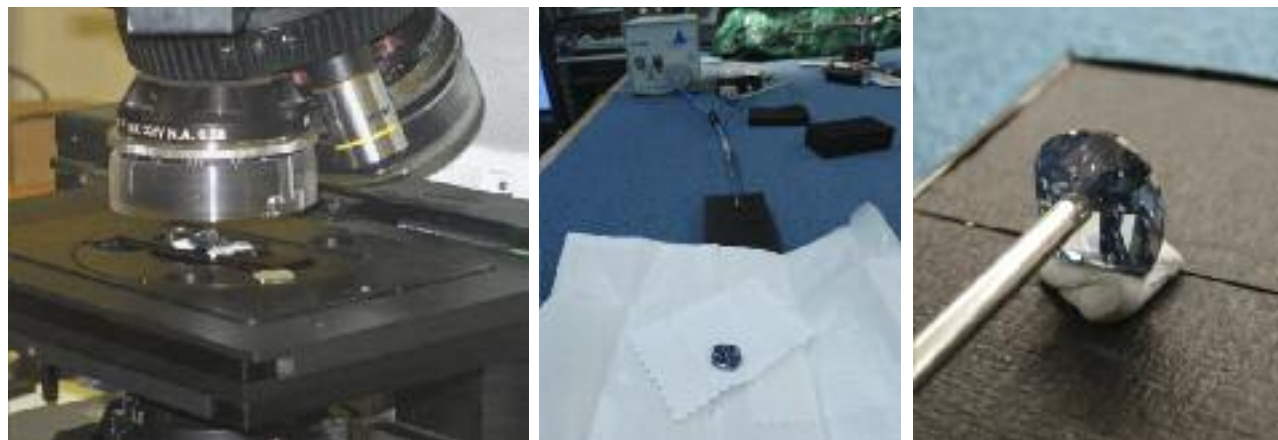
Figure 2. Left: The Blue Moon is shown under the microscope of the FTIR spectrometer, which identified it as a type IIb diamond with an uncompensated boron concentration of 0.26 \pm 0.04 ppm. Center: A view of the Blue Moon and the phosphorescence equipment, composed of a deuterium lamp source, a spectrometer, and fiber optics. Right: The Blue Moon under the tip of a fiber-optic bundle used for the phosphorescence experiments. All analyses were conducted at the Smithsonian Institution. Please indicate the photographer(s).
