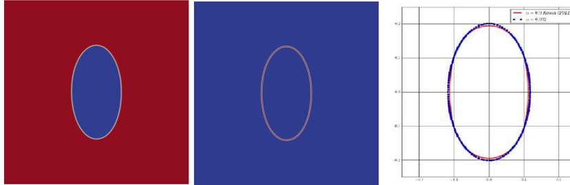
Figure 9: Level set function, Dirac function and the reference solution for  $\eta = 0.9$
