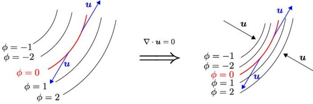
Figure 3: Principle of the inextensibility by elastic force [36]
