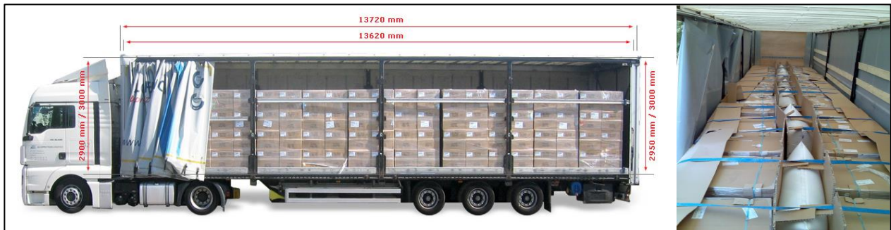
Figure 13. Palletized cases in semi-trailers with highly different space filling rates
