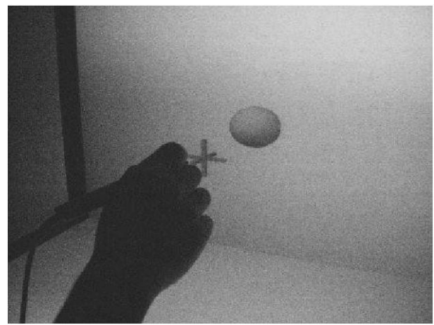
Figure 3. Direct manipulation: the cursor used to interact with the objects (cross) is as close as possible to the user's hand.
