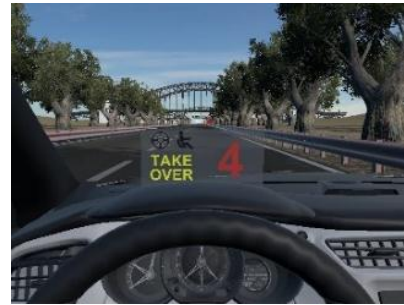
Fig. 5 – Take Over Request displayed on the HUD
