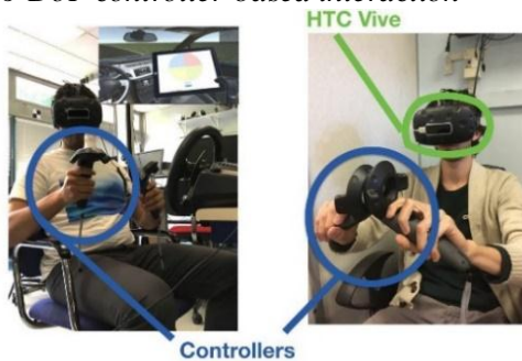
Fig. 3 – 6-DoF controller-based interaction
