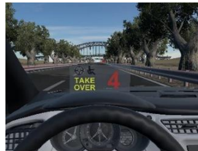
Fig. 5 – Take Over Request displayed on the HUD
