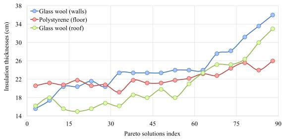
Figure 8 Evolution of the insulation thicknesses for decreasing GHG emissions (Pareto solutions)
