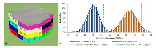
**Figure 8** (a) Thermal zones of the building (design interface of the simulation tool *Pleiades+Comfie*). (b) Heating loads distributions for two temperature setpoints corresponding to measuremements before and after renovation.
