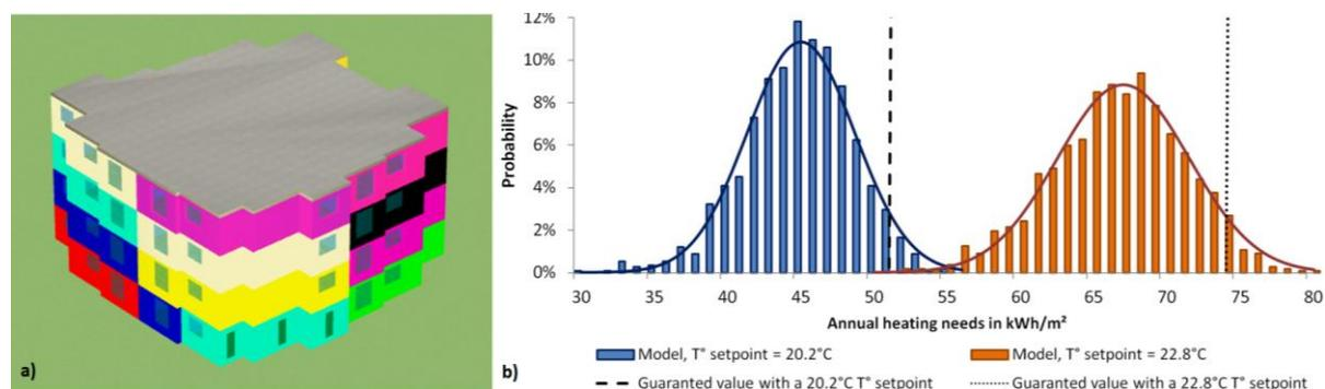
**Figure 8** (a) Thermal zones of the building (design interface of the simulation tool *Pleiades+Comfie*). (b) Heating loads distributions for two temperature setpoints corresponding to measurements before and after renovation.
