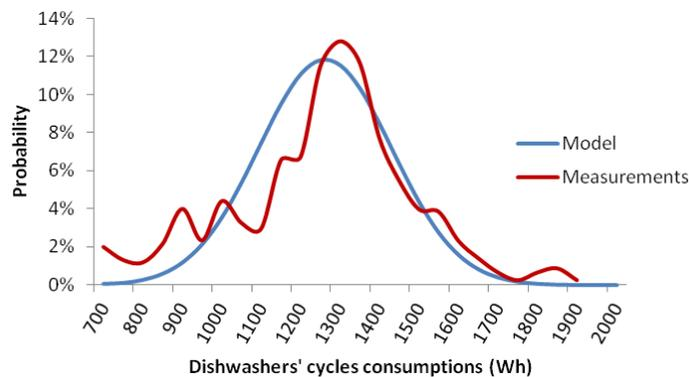
**Figure 4** Comparison between modeled and measured cycles consumptions.
