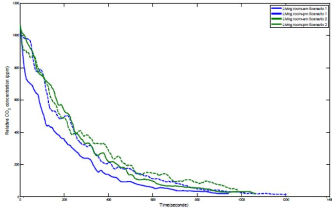
Figure 5: Relative CO<sub>2</sub> concentration in the living room during CO<sub>2</sub> decay test
