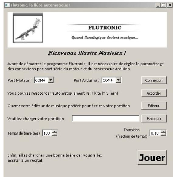
Figure 7: The musical interface — From top to bottom: The first line of buttons is used for communication setup — The second line is used for starting the calibration process — The third line is used for launching the score's writing software — The fourth line is used to load a score — The fifth line is used for setting tempo and time transition of playing — The last button is used to launch the play.
