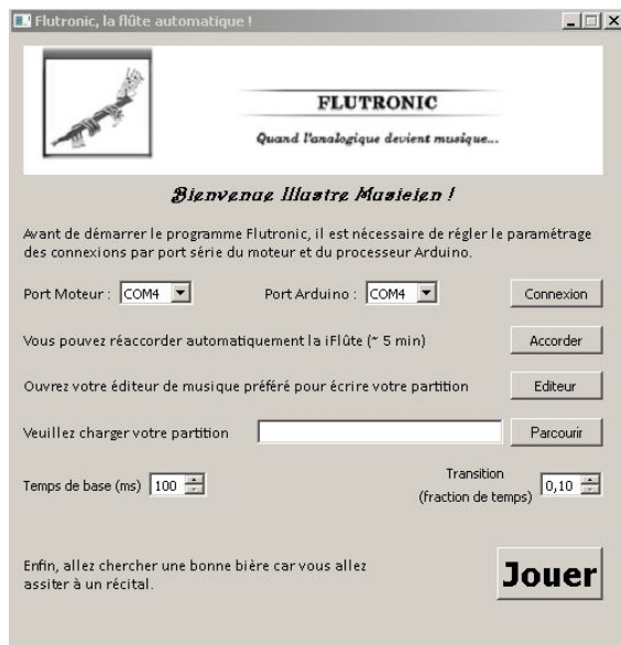
Figure 7: The musical interface — From top to bottom: The first line of buttons is used for communication setup — The second line is used for starting the calibration process — The third line is used for launching the score's writing software — The fourth line is used to load a score — The fifth line is used for setting tempo and time transition of playing — The last button is used to launch the play.
