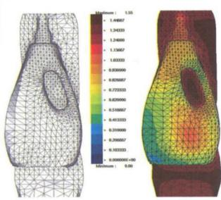
**Figure 8.** (top) Shape and meshing of the membrane at different steps of simulation of the extrusion; (bottom) Final mesh and thickness distribution in the bottle (Bellet et al.[34])
