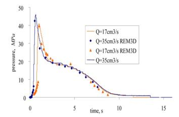
**Figure 7.** Pressure as a function of time in the cavity during the entire injection cycle for two different flow rates, the polymer is a polystyrene (Silva et al.[11]).
