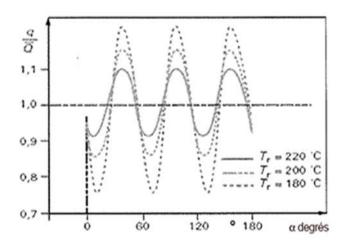
**Figure 5.** Influence of the thermal regulation of the die shaft on the polymer flow distribution at film-blowing die exit.. q is the local flow along the circumference of the die,  $\bar{Q}$  is the average flow rate (Vergnes et al.[12];Agassant and Vergnes [13])
