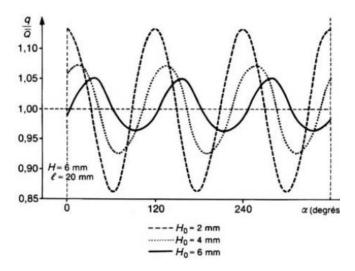
**Figure 4.** Influence of the initial depth of the channel  $H_0$  on the polymer flow distribution at film-blowing die exit. q is the local flow along the circumference of the die,  $\bar{Q}$  is the average flow rate ( Vergnes et al.[12];Agassant and Vergnes [13]).
