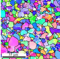
**Figure 6**. EBSD grain map from 6mm behind the pin in the location where the tool was retracted, at the end of the experiment. Average recrystallized grain size at this location was 7 mm, compared to an average grain size of 25 mm in the base material.
