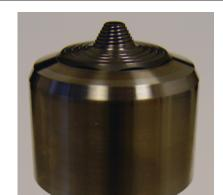
Figure 2. Friction stir processing tool, with convex shoulder and conical pin.
