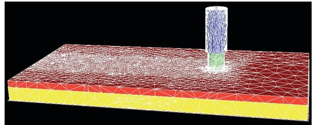
**Figure 3.** Model of friction stir processing of 304L plate. The tool (green) is embedded in the 304L plate (red). A constant temperature boundary condition of 19°C is imposed by the tool holder (blue) on the shank of the tool. The backing plate (yellow) is supported by a rigid support with a constant temperature boundary condition of 50°C.
