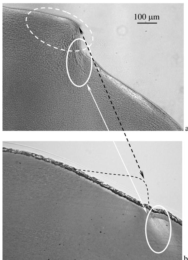
Figure 8: optical microscopy observation under polarization with a lambda plate of thin cuts ( $e = 5 \mu\text{m}$ ) from injected parts before (a) and after polishing (b)
