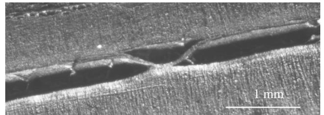
Figure 7: Macrograph of a crack on the surface after immersion inside solvents
