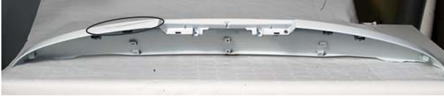
Figure 2. Bottom view of a spoiler (the defective zone is bordered)
