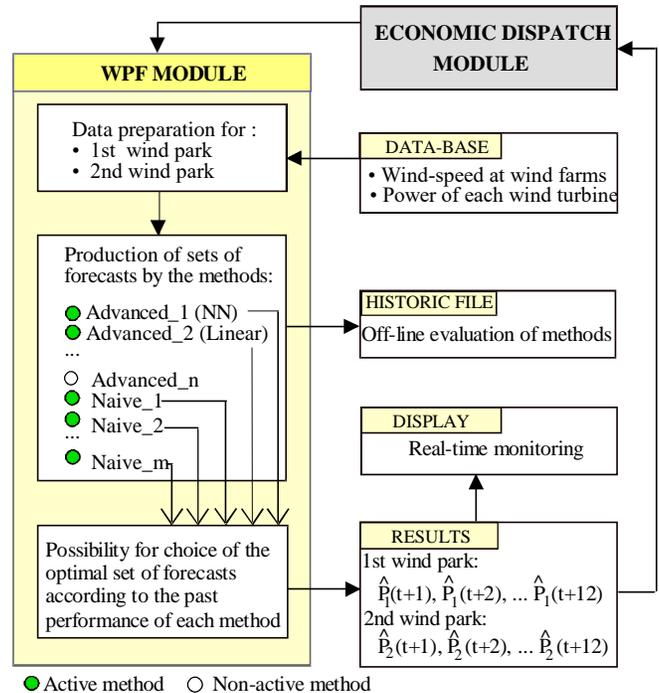
Fig. 4 : Flow-chart of the WPF module operation.
