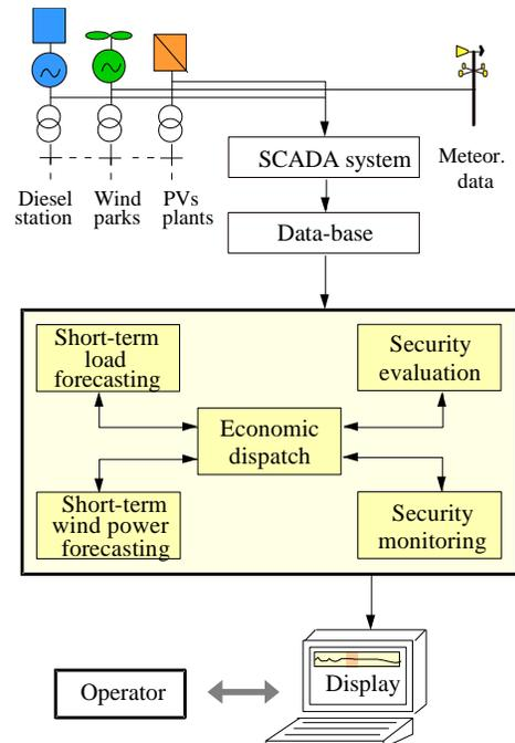
**Fig. 3 :** The architecture of the pilot control system
