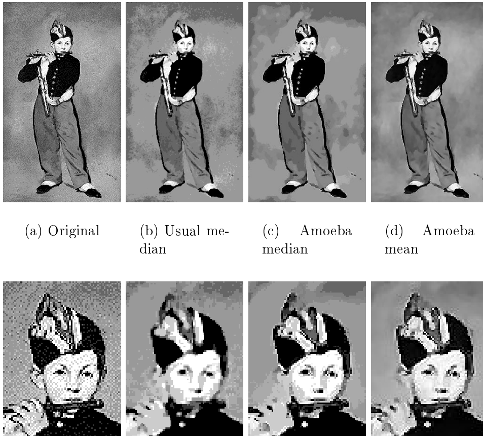
Fig. 7. Results of a “classic” median filtering and two amoeba-based filterings: a median and a mean on Edouard Manet’s painting “Le fifre”.
