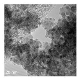
Figure 1. TEM image of a Pt/Sb-doped SnO<sub>2</sub> aerogel obtained from method A
