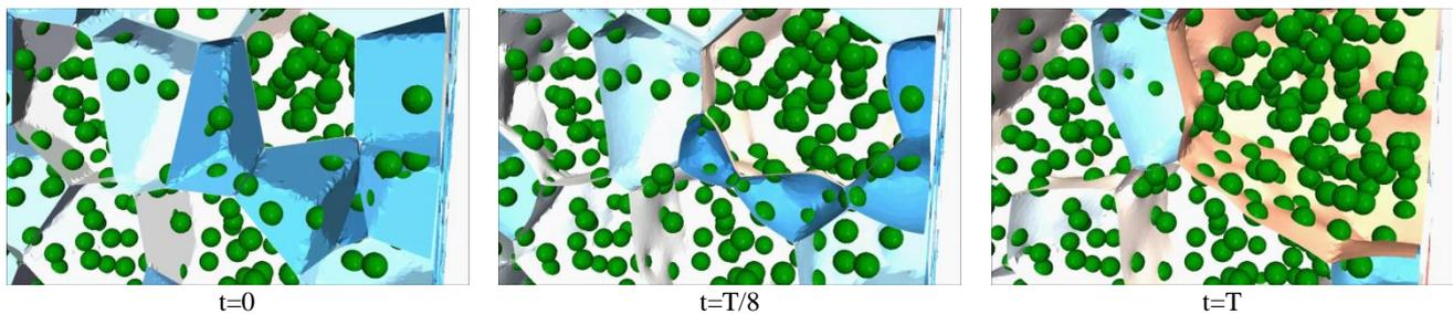
Figure 5. A 3D grain growth simulation for Inconel™ 718. The green spheres represent the precipitates.
