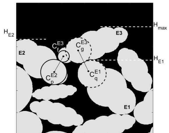
Figure 6. Placement of the ellipse E3 on E1 and E2. The corresponding pairs of circles  $C_q^{E1} - C_g^{E3}$ ,  $C_p^{E2} - C_f^{E3}$  in contact and ellipses heights ( $H_{E1}$ ,  $H_{E2}$  and  $H_{max}$ ) are shown.
