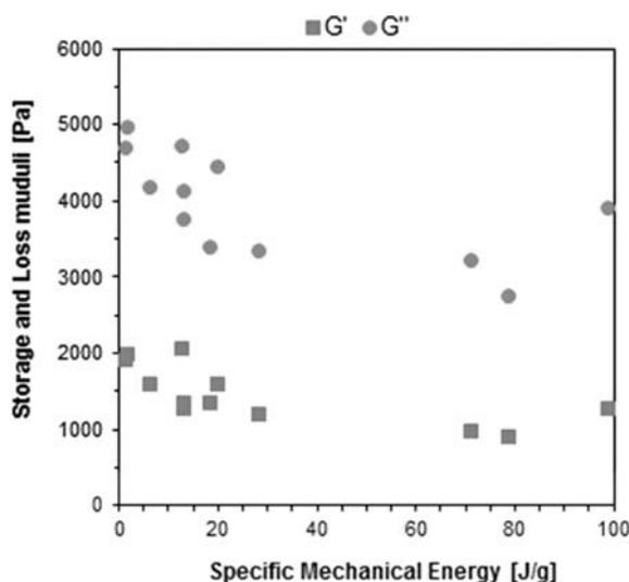
FIG. 5. Storage and loss moduli at 0.1 rad/s as a function of the SME for plasticized cellulose acetate prepared with the four different processing tools. [Color figure can be viewed at [wileyonlinelibrary.com](http://wileyonlinelibrary.com)]
