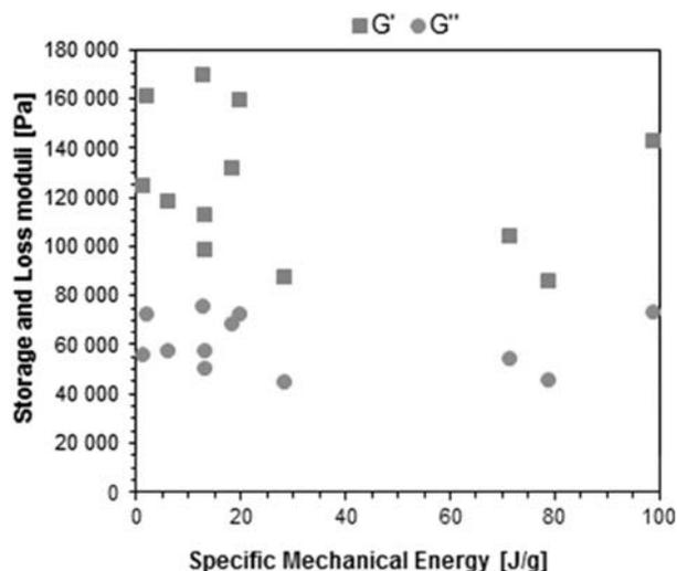
FIG. 4. Storage and loss moduli at 100 rad/s as a function of SME for plasticized CA prepared with the four different processing tools. [Color figure can be viewed at [wileyonlinelibrary.com](http://wileyonlinelibrary.com)]
