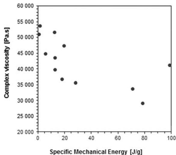
FIG. 6. Complex viscosity measured at 0.1 rad/s as a function of the SME. [Color figure can be viewed at [wileyonlinelibrary.com](http://wileyonlinelibrary.com)]
