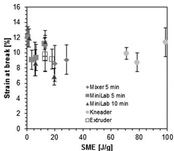
FIG. 8. Strain at break as a function of the SME. [Color figure can be viewed at [wileyonlinelibrary.com](http://wileyonlinelibrary.com)]
