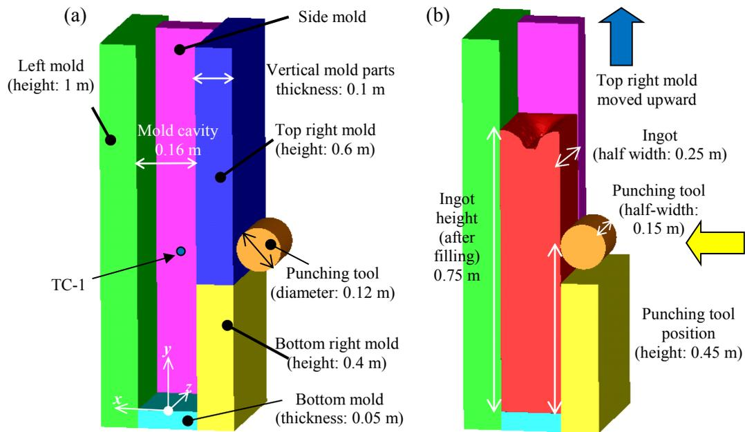
**Figure 1.** Schematic of the ingot punching test developed at Nippon Steel & Sumitomo Metal Corporation showing (a) initial state and (b) punching stage after the top right mold was removed. The configuration shown is half of the setup, considering symmetry with respect to the central transverse section through the whole system. A thermocouple (TC-1) is placed at coordinates  $(0, 0.43, 0.06)$ , with reference frame centered at the top surface of the bottom mold plate.
