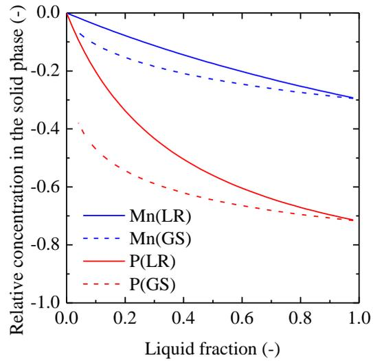
**Figure 16.** Relative variation of average solute concentration in the solid phase as a function of the liquid fraction. The dependence is plotted for solutes Mn and P, and for two microsegregation models: (LR) lever rule and (GS) Gulliver-Scheil. The relative variation of the concentration in the solid phase is calculated as  $(w_{s,i} - w_{i0})/w_{i0}$  where  $w_{i0}$  is the concentration of solute  $i$  at the beginning of solidification.
