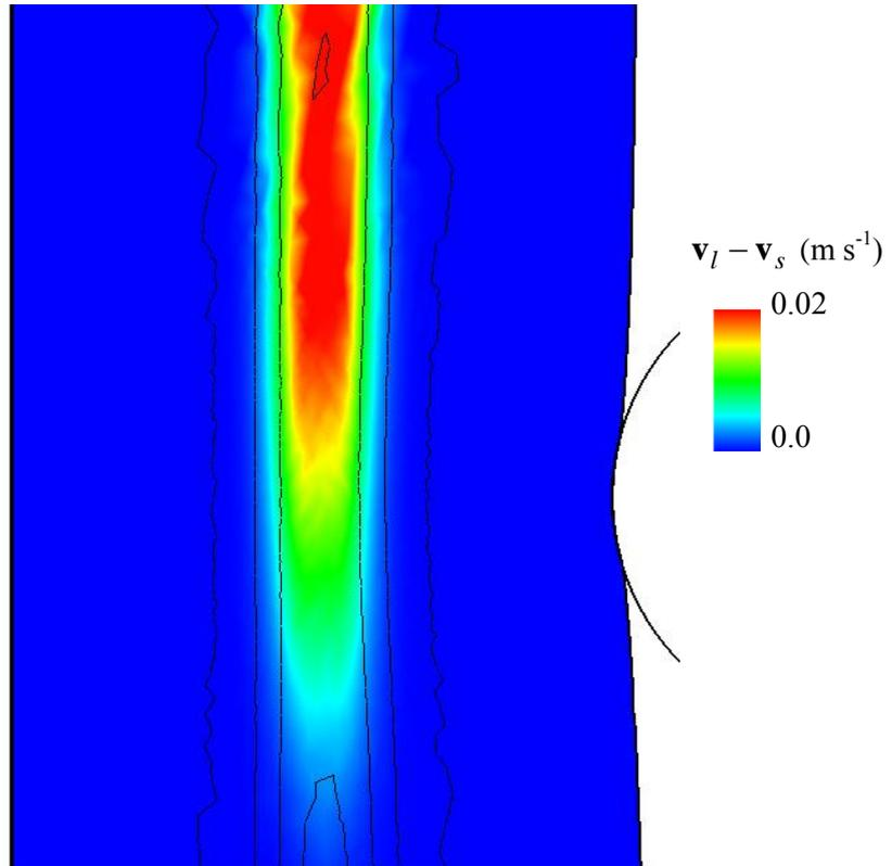
**Figure 12.** Relative velocity field along vertical direction with the isolines of liquid fraction 4 s after the start of punching.
