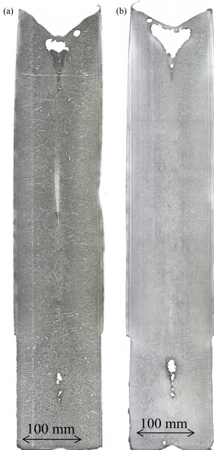
**Figure 2.** Micrograph at central transverse section of (a) N-1 and (b) N-9 ingots. Macro-segregation is qualitatively revealed by the variations of the grey level. The print of the punching tool is visible on the right hand side in these images.
