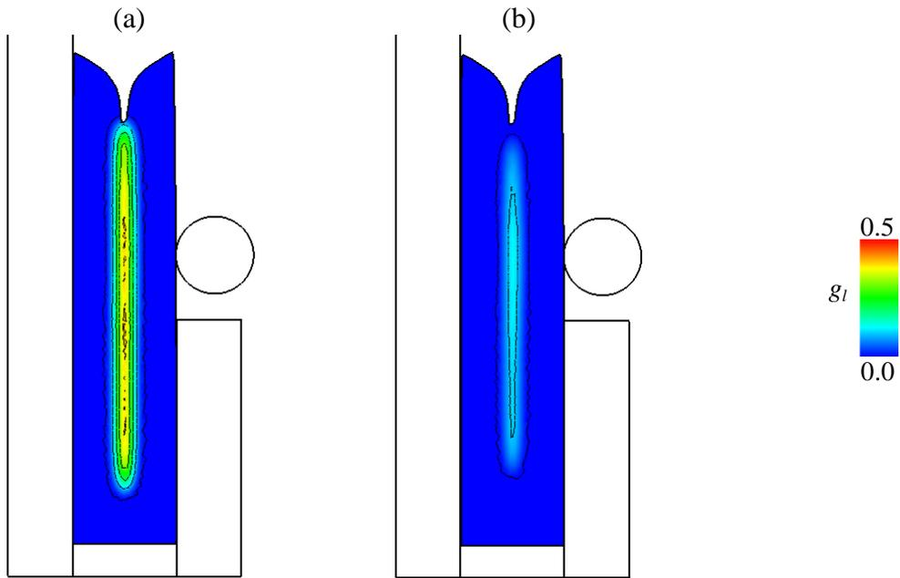
**Figure 7.** Calculated shape of the ingot and distribution of the liquid fraction just before punching (a) at time 792 s (corresponding to trial N-1) and (b) at time 881 s (corresponding to trial N-9).
