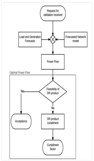
Figuare 17: OLV diagram
