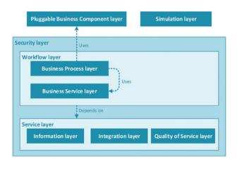
Figure 34: Architecture of the USEF reference implementation.
