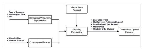
Figure 19: The different modules of the Commercial Aggregators
