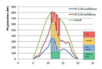
Figure 4: Updated intra-day forecasts can be used to allocate production to different markets.
