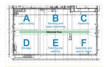
Figure 30: Schematic Overview of Material Flow and Factory Layout
