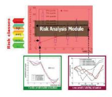
Figure 1: Example of a probabilistic forecast for a wind farm. Ramps forecasting based in ensemble NWPs, Illustration of the prediction risk index concept based on ensembles.
