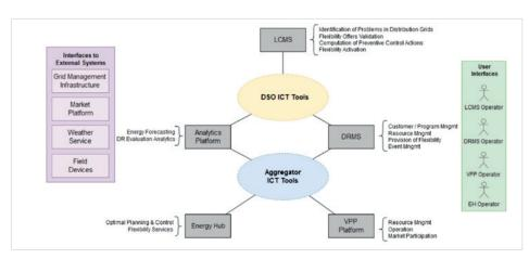
Figure 14: The SmarterEMC2 High Level Conceptual Architecture
