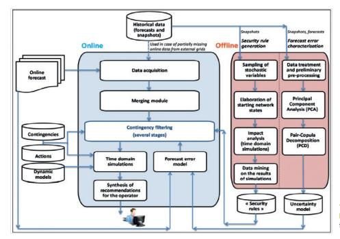
Figure 6: Overall work flow of the iTESLA platform
