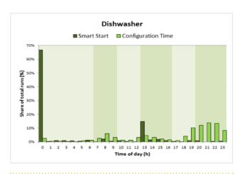
Figuare 20: Shifting of dishwasher consumption without control (light green) towards the night time and afternoon with PV (dark green)
