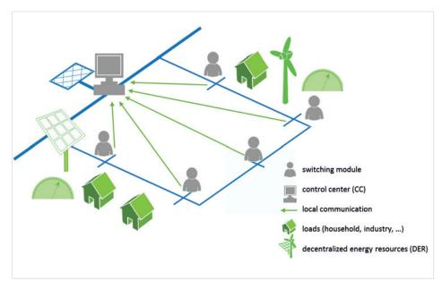
Figure 7: The basic principle
