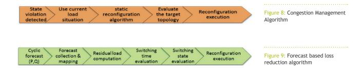
To get more information about the grid reconfiguration algorithm, please refer to the "grid reconfiguration algorithm" spotlight of the GRID4EU German Demonstrator.
