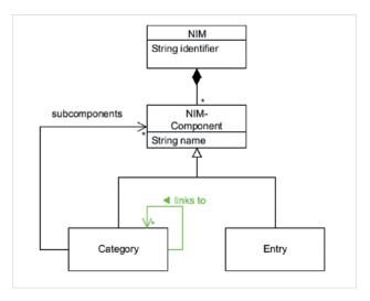
Figuare 27: The main parts of the NIM. The concept of scopes as well as the abstraction of concrete data is shown.
