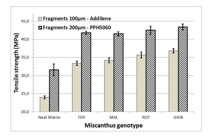
Figure 6: Ultimate tensile strength for composites reinforced with 30% wt of fragments
