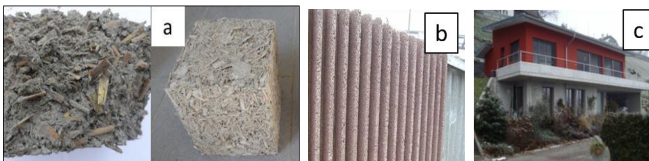
Figure 5. a) Miscanthus-based mix and block (author's work) and b) a miscanthus based noise barrier and (c) a house built with miscanthus concrete [106]. With authorisation of asbl ValBiom, Croix du Sud 2, bte 11, 1348 Louvain-la-Neuve, Belgium.
