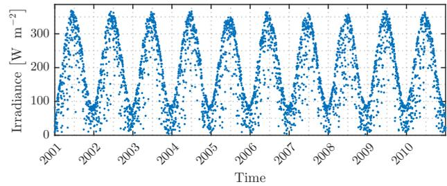
**Figure 1.** The ten year time-series of SSI under study, spanning 2001 through 2010. Each point corresponds to a daily mean of irradiance. Time markers on the abscissa denote the start of the corresponding year.
