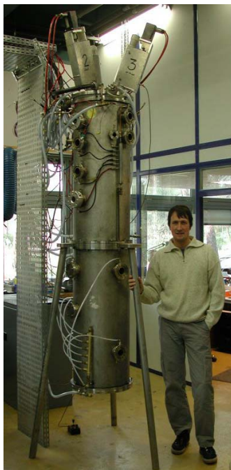
Figure 1: Overall picture of the 3-phase AC plasma reactor (2 meters high).
