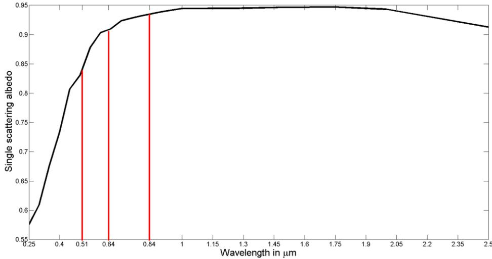
**Figure 4:** Single scattering albedo of mineral dust in the visible and near infrared according to OPAC. The 3 red lines represent the central wavelength of the channels VIS0.5, VIS0.6 and VIS0.8 of the FCI.
