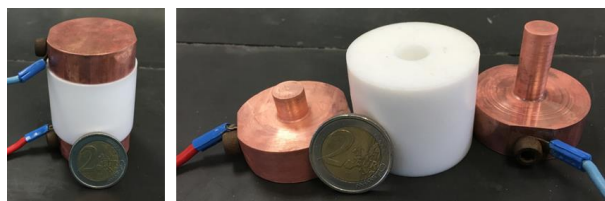
Fig 1 Homemade conductivity cell picture assembled (left) and disassembled (right)
