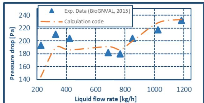
Fig. 12 Influence of liquid flow rate on the pressure drop
