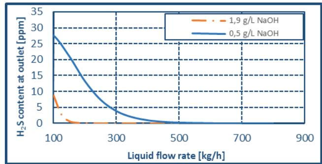
Fig. 11 Influence of the liquid flow on the absorption of H<sub>2</sub>S
