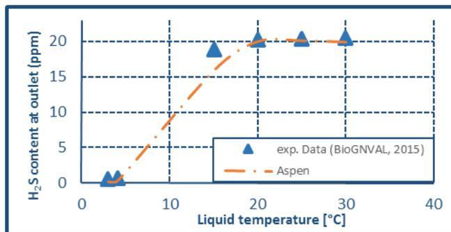
Fig. 14 Influence of the temperature of liquid in the absorption of H<sub>2</sub>S
