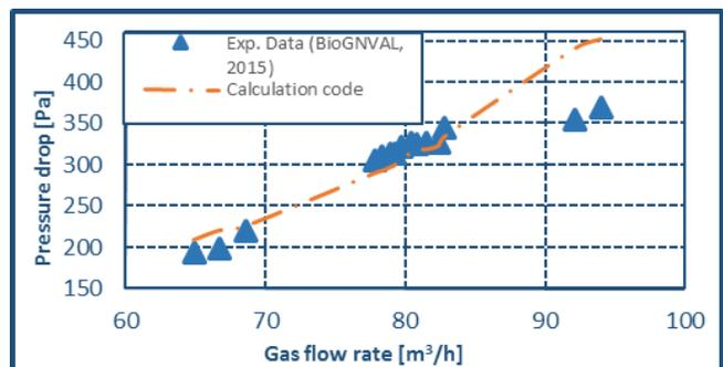
Fig. 13 Influence of gas flow rate on the pressure drop
