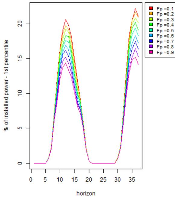
Figure 3: level of the worst errors of PV production along years 2007 up to 2012, as a function of the forecasting time horizon, and the spatial dispersion of PV systems ( $F_p=0.1$  represents a concentration of solar panels only on the best sites and  $F_p=1$  represents a uniform distribution over France). Only the forecasts issued at 00:00 are used in this Figure.
