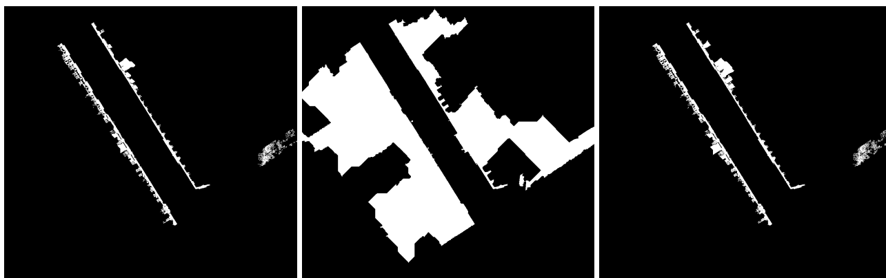
(a) Façade markers F_{mark} . (b) Reconstruction by dilation R_{Gc}^{\delta}(F_{mark}) . (c) Attribute controlled reconstruction A_{\lambda_M}(F_{mark}) .
