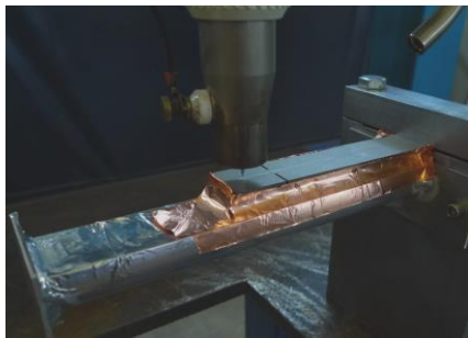
Figure 1: Hot cracking test: a) geometry of plate specimens ; b) experimental set-up showing clamping and protection against oxidation on the lower side of the plate ; c) example of a crack fully developed throughout the weld bead (test 4 of Table 2).
