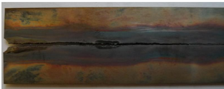
Figure 1: Hot cracking test: a) geometry of plate specimens ; b) experimental set-up showing clamping and protection against oxidation on the lower side of the plate ; c) example of a crack fully developed throughout the weld bead (test 4 of Table 2).
