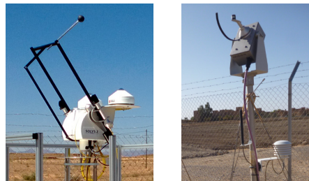
FIGURE 2. On the left the thermal sensor station of Missouri, Morocco. On the right one can see the RSI in Erfoud, Morocco.
