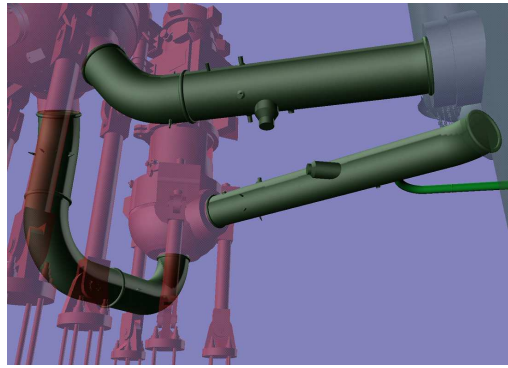
Fig. 5 : MCL location into the reactor vessel.
