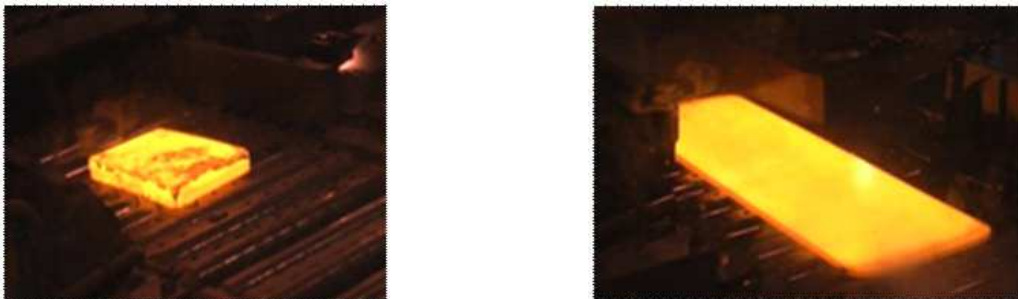
Fig. 2 : Hot rolling of thick plate.
