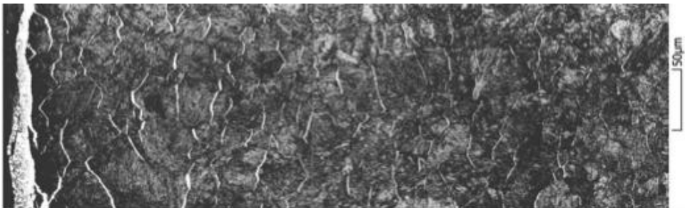
Figure 10: Micrograph showing the white layer and the diffusion layer after nitriding (Arts et Metiers ParisTech Aix-en-Provence)
