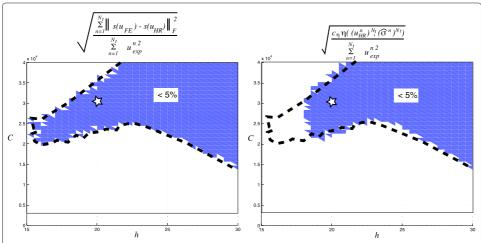
**Figure 6** Error prediction on outputs. On the left, in blue, the reference validity domain  $\mathcal{D}_V$  over the parameter space  $\mathcal{D}$ , on the right the approximate one  $\widetilde{\mathcal{D}}_V$ . The white star is located at the sampling point  $\mu^1$ . The black dashed line is the limit of the reference validity domain defined by an error on the outputs lower than 5%.
