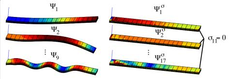
**Figure 3** Empirical modes. Some POD modes: on the left for displacements and on the right for admissible stresses.
