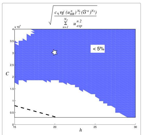
**Figure 8** Error prediction on outputs in case of non-zero Dirichlet boundary condition. In blue, the approximate validity domain  $\widetilde{\mathcal{D}}_V$ . The white star is located at the sampling point  $\mu^1$ . The black dashed line is the limit of the reference validity domain defined by an error on the outputs lower than 5%.
