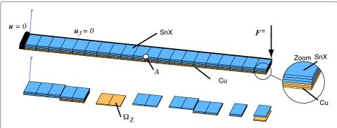
**Figure 2** Meshes. On the top, we show the boundary condition and the mesh of the FE model. On the bottom, we show the RID involving 31 elements of the original mesh.
