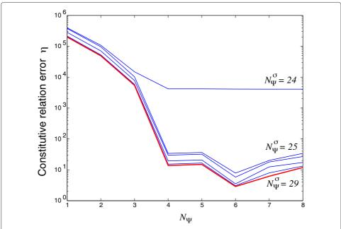
**Figure 4** Convergence of the error estimator. The constitutive relation error depends on both displacement approximation and admissible stress approximation. Here,  $\mu = \mu^1$ .
