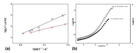
Figure 7. (a) Arrhenius plots resistivity for BCY15 (o) with 12% porosity and YDC15 (d) and (b) frequency dependence of C' in BCY15 with different porosity and the same pore former.
