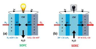
Figure 3. The (a) SOFC and (b) SOEC modes.
