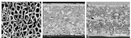
Figure 9. BSE-SEM images of (a) laminated nickel foams at 1 kg cm<sup>-2</sup>, (b) screen-printing Ni-foam cell, (c) dip-coated Ni-foam cell.
