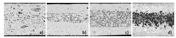
Figure 5. Central membrane porosity sintered at 1400 °C for 5 hours: (a) no-graphite, (b) 10 vol.% graphite, (c) 20 vol.% graphite and (d) 30 vol.% graphite.
