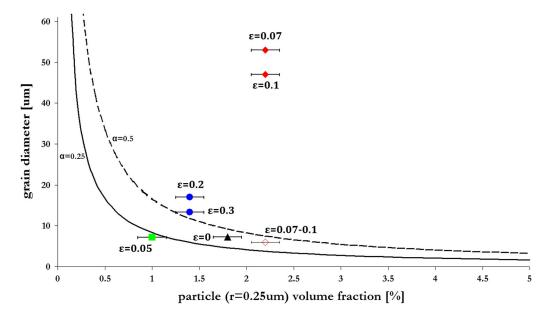
Fig. 5—Comparison of grain size predicted by Eq. [1] and values measured on samples characterized by different initial levels of strain  $(0 < \varepsilon < 0.3)$  after  $\delta$  sub-solvus annealing for 2 h. The empty square corresponds to the minor population of bimodal microstructures in samples  $\varepsilon = 0.07$  and  $\varepsilon = 0.1$ . Note: the  $\delta$  phase fraction is measured before annealing.
