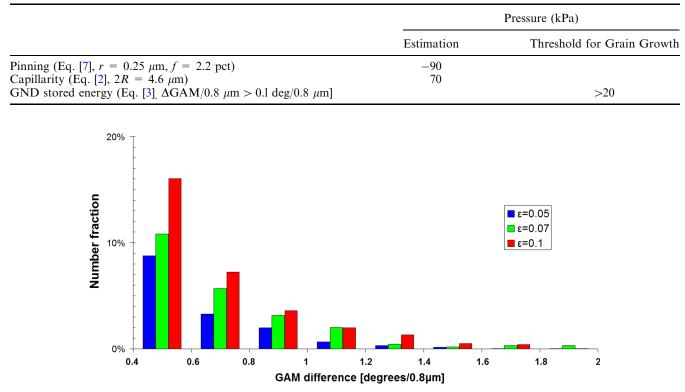
Fig. 15—Histogram of the fraction of grain and twin boundaries separating two crystals with a fixed GAM difference in samples strained up to  $\varepsilon = 0.05$  and  $\varepsilon = 0.1$ . The fraction of boundaries corresponding to a GAM difference lower than 0.4 deg/0.8  $\mu$ m is not displayed.
