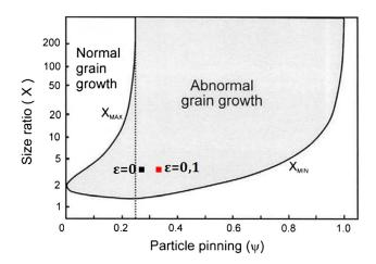
Fig. 13—Plot from<sup>[8]</sup> of minimum grain size ratio (X) to trigger abnormal grain growth as a function of Smith–Zener pinning ( $\psi$ ): microstructures of samples  $\varepsilon = 0$  and  $\varepsilon = 0.1$  fall in the area where abnormal grain growth is possible.
