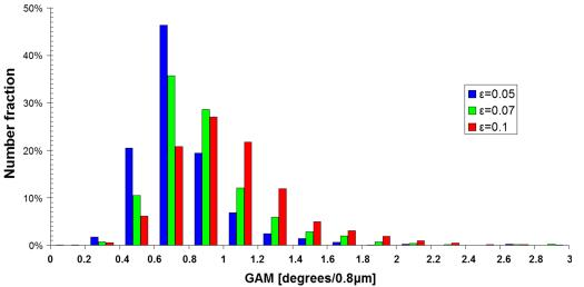
Fig. 16—GAM distribution (number fraction) of all crystals (*i.e.*, individual GAM values are calculated for each crystal in a twinned grain) in samples strained up to  $\varepsilon = 0.05$  and  $\varepsilon = 0.1$ .
