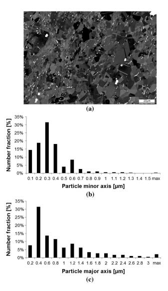
Fig. 3—Distribution of the  $\delta$  phase in the initial microstructure: (*a*) BSE image showing the  $\delta$  phase as small white particles and few carbides (NbC) as bigger particles, (*b*) minor axis, and (*c*) major axis particle number fraction.
