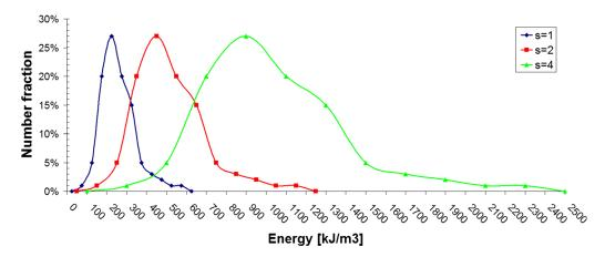
Fig. 17—Strain stored energy distribution of sample  $\varepsilon = 0.1$  before annealing. The parameter s is introduced to take into account the energy contribution of statistically stored dislocations.
