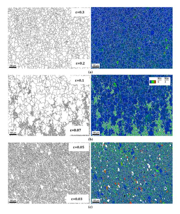
Fig. 9—Microstructures after  $\delta$  sub-solvus annealing for 2 h in samples characterized by different initial levels of strain: (a)  $\varepsilon = 0.3$ , (b)  $\varepsilon = 0.1$ , (c)  $\varepsilon = 0.05$ . Left images display EBSD maps only with grain boundaries in black, and right images show grain orientation spread (GOS) maps with grain boundaries in white and twins in black. Note: white grains have GOS values higher than 3 deg.
