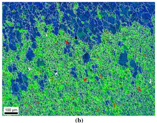
Fig. 12—Microstructure after  $\delta$  sub-solvus annealing for 15 min of sample  $\varepsilon = 0.1$ -bis. EBSD map showing grain boundaries in black and twins in gray (*a*) and related map of grain orientation spread (GOS) maps with grain boundaries in white and twins in black (*b*). Note: white grains have GOS values higher than 3 deg.
