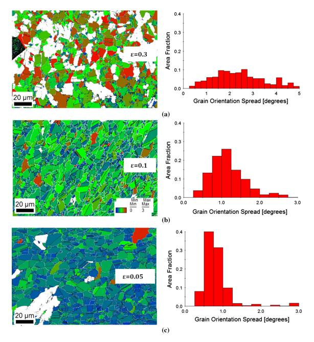
Fig. 7—Grain orientation spread (GOS) maps and distributions (area fraction) in the strained samples before annealing as a function of local equivalent strain: (a)  $\varepsilon = 0.3$ , (b)  $\varepsilon = 0.1$  and (c)  $\varepsilon = 0.05$ . In GOS maps, the grain boundaries are in white, the twins are in black, and white grains have GOS values higher than 3 deg.
