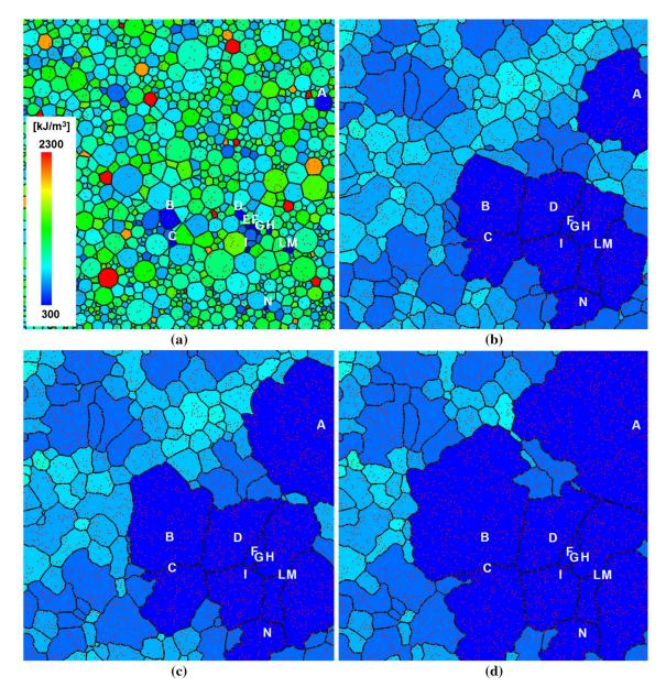
Fig. 19—Evolution of a microstructure with an initial energy distribution equivalent to that of Fig. 17 (s = 4) and a particle fraction equivalent to 4 pct after annealing at 1258 K for different times: initial microstructure (a), 300 s (b), 600 s (c), and 900 s (d).
