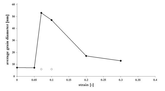
Fig. 11—Influence of local strain on final grain size after  $\delta$  sub-solvus annealing for 2 h in samples characterized by different initial levels of strain. Empty squares correspond to the minor population of bimodal microstructures.
