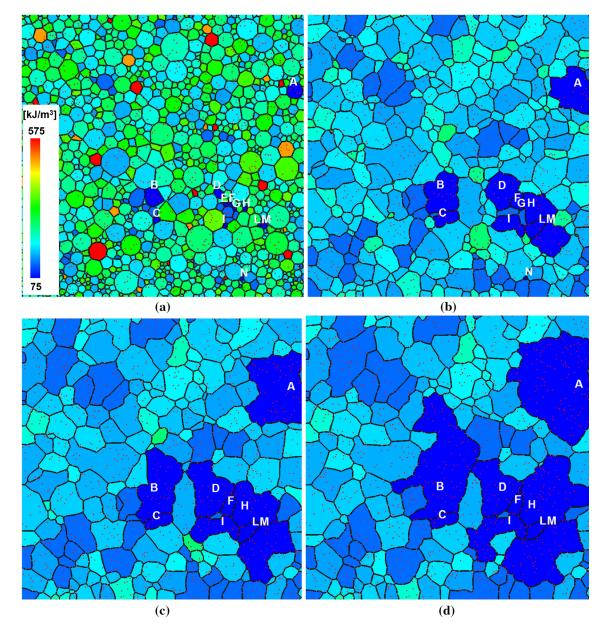
Fig. 21—Evolution of a microstructure with an initial energy distribution equivalent to that of Fig. 17 (s = 1) and a particle fraction equivalent to 2 pct after annealing at 1258 K (985 °C) for different times: initial microstructure (a), 300 s (b), 900 s (c), and 3300 s (d).
