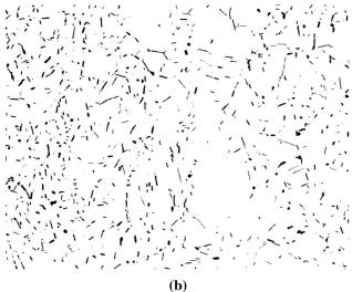
Fig. 6—Grain bigger than the Smith–Zener limit in the initial microstructure after  $\delta$  sub-solvus annealing for 2 h: (a) BSE image, (b)  $\delta$  phase filtered.
