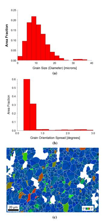
Fig. 2—Initial microstructure properties determined by EBSD measurements. Grain size distribution histogram (*a*). GOS distribution histogram (*b*). EBSD map (*c*): grain boundaries in white, twins in black, and grain colors related to GOS values (white grains have higher GOS values than 3 deg) (Color figure online).
