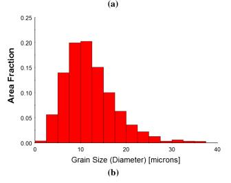
Fig. 4—Grain size distribution determined by EBSD in the initial microstructure after  $\delta$  sub-solvus annealing for 2 h: (*a*) grain boundaries in black (twins excluded), (*b*) grain size distribution histogram.
