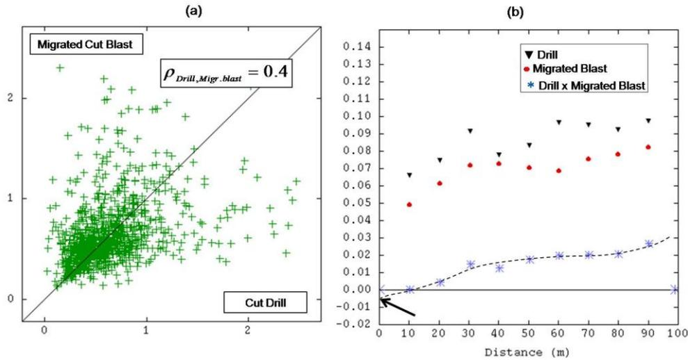
**Figure 5.** (a) Scatter diagram between migrated blasts and drills; (b) Direct variogram of migrated blasts (black triangles), corresponding drills (red points) and cross-variogram of both (blue stars). The cross variogram reveals a tiny negative nugget effect with no comparison with the drill or blast ones
