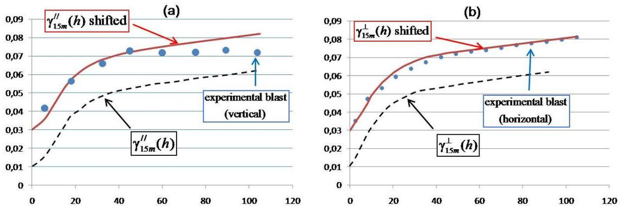
**Figure 4.** In blue, the points of the experimental blast variogram; dotted line, the theoretical model for the blasts deduced from the drills; in red, the theoretical model with a more realistic nugget effect (a) Theoretical regularization parallel to the vertical blast variogram (b) Theoretical regularization perpendicular to the horizontal blast variogram.
