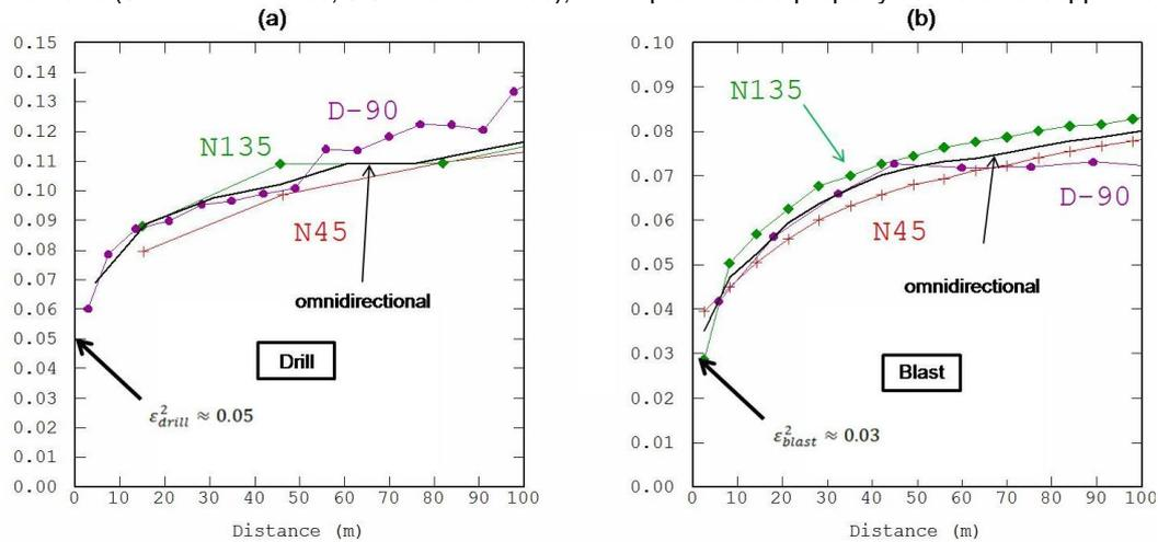
**Figure 2. (a) Drill hole copper grade variogram; (b) Blast copper grade variogram. Three directions are represented, 45° North (N45), 135° North (N135), and vertical (D-90). Black continuous line is the isotropic variogram**
