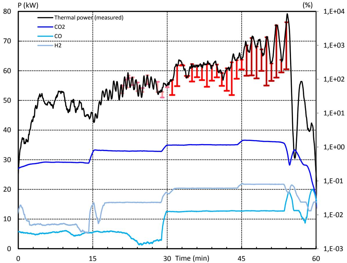
Figure 4: Total measured thermal power (black) , CO<sub>2</sub>, CO and H<sub>2</sub> volume percentage (from dark to light blue). The colored arrows represent the difference between the total measured thermal power and the measured electric power at different biomass injection rate 1.1 kg.h<sup>-1</sup>, 2.2 kg.h<sup>-1</sup> and 3.3 kg.h<sup>-1</sup> (from light to dark red).
